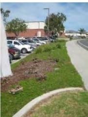
GSA installed jute mesh to stabilize the slope at the Telephone Road building, along with new mulch which suppresses weed growth and reduces the need for herbicides and pesticides. New mulch retains soil moisture, resulting in a 30% savings in water efficiency for the sprinkler nozzles which were exchanged. The sprinkler nozzles apply water at a slower rate and with less misting to reduce water loss from runoff, drift, and evaporation.
